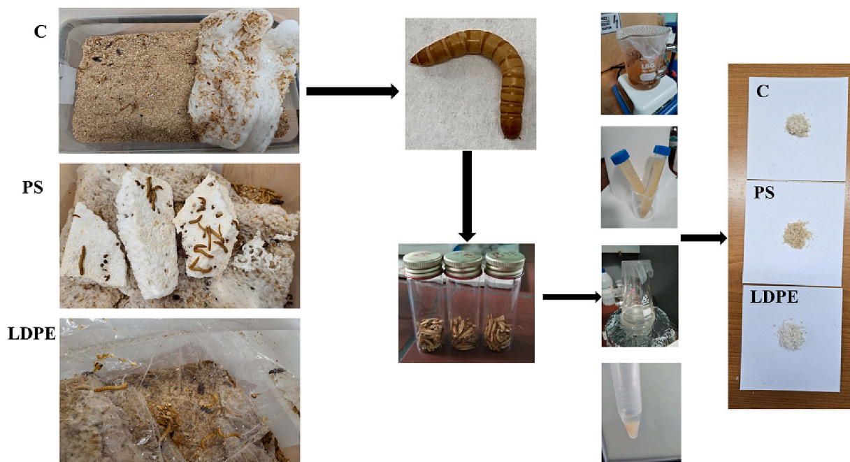
Fig. 1. Schematic illustration of extraction steps of chitin from freeze dried exoskeletons of Tenebrio molitor larvae fed with wheat bran (C-control group), wheat bran with added polystyrene (PS group), or plastic kitchen wrap (LDPE group).
