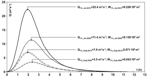
Fig. 4 Computed hydrographs of maximal discharges into the Kaljavi and Jelezovac streams (under conditions before and after restoration of the "blue-green" corridors).
