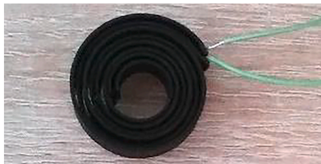
Fig. 4. The photograph of the fabricated rolled capacitor with added contacts.
