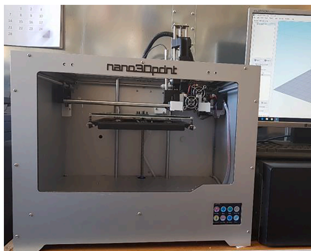
Fig. 3. 3D Multimaterials printer, A2200, manufactured by Nano3Dprint.
