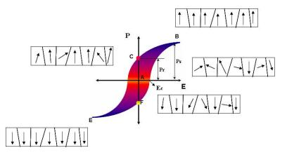
Fig. 1. A typical P-E hysteresis loop in ferroelectrics[3]
