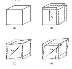
**Fig. 3.** Unit cells of the four phases of  $BaTiO_3$ :(a)Cubic, stable above 120 °C, (b)Tetragonal, stable between 120 °C and 5 °C, (c)Orthorhombic, stable between 5 °C and -90 °C, (d)Rhombohedral, stable below -90 °C,
