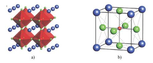
Fig. 2. Cubic perovskite-type structure ABO<sub>3</sub> [8]
