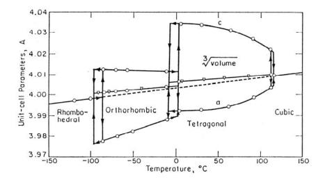
Fig. 5 Lattice constants of BaTiO<sub>3</sub> as function of temperature [1]
