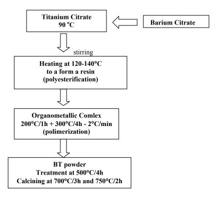
Fig. 7 The flow chart for the Pechini process of BaTiO<sub>3</sub> [26]
