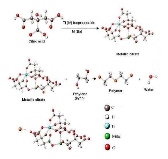
Fig. 6 Polymeric precursor method-Pechini process [26]
