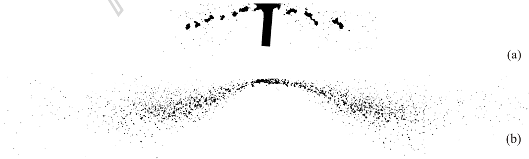
Fig. 1. Fragmentation snapshots corresponding to the moment of projectile arrest (a) or full fragmentation (b) for two striking velocities: (a) 0.75 km/s and (b) 3 km/s. Note how the nanoprojectile at striking velocity approaching the hypervelocity impact threshold dissolves in a cloud of particles as the entire projectile is being shattered. This lateral “splash” of the escaping high-temperature debris is similar to the breakup of liquid droplets colliding with a wall as discussed in [28] in connection with the enhanced ductility of fragmenting plastic materials due to the temperature-driven reduction of the shear resistance.
