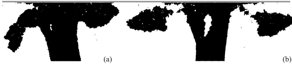
Figure 1. Snapshot of two severely deformed configurations of a projectile \bar{d} = 57 ( m = 26047 ; the total mass given in number of atoms) following an impact at (a) v_i = 0.465 km/s and (b) v_i = 0.475 km/s. (a) The arrested projectile with no large fragments; the corresponding snapshot time exceeds the effective arrest time approximately three times ( \approx 3 \cdot t_A ). Note the nucleation of diffuse voids and initiation of nanoscale cracks by their coalescence. (b) The separation of the two largest fragment (followed by the projectile arrest shortly after) with notable growth of a blunted vertical crack whose propagation is stopped eventually. (The projectile stumps are cut to emphasize the proximal-end details. The stump disappears with the complete projectile fragmentation which is, within the present simulation framework, roughly identified with the striking velocity range of 2-3 km/s (Mastilovic, 2015). Furthermore, to get a feeling for the striking velocities used in the present investigation, the velocity of longitudinal elastic wave propagation of the LJ solid used herein is approximately 4.3-4.4 km/s which is within 5-10% of the reported values for tungsten (Mastilovic, 2016).)
