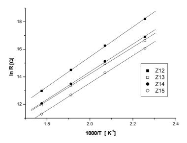
Fig. 2. Arrhenius plots of resistance vs. temperature for Z12, Z13, Z14 and Z15 varistors.
