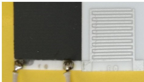
Fig. 1 Iron manganite thick film sample (left) and alumina substrate with test PdAg electrodes (right)
