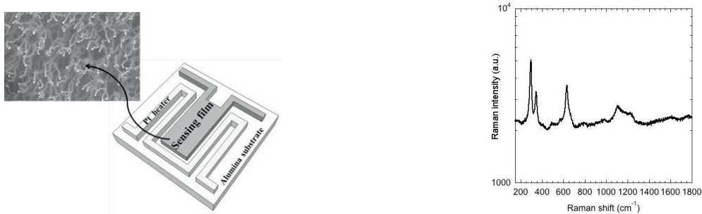
Figure 1: (Left) SEM image of nanostructured p-type thin film of Cu-Al-Oxide sensing layer is deposited by RF sputtering with schematic diagram of sensing thin film. (Right) Raman signal of aged sensing thin film used for sensor and the CuO monoclinic phase can be detected.
