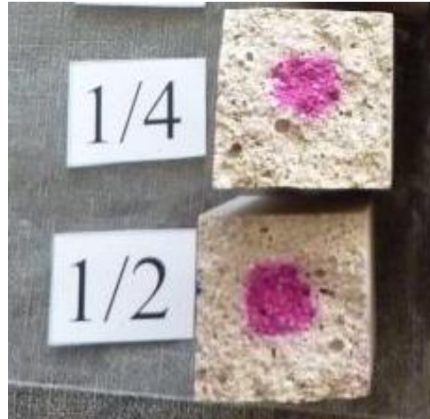
Figure 2: Carbonation identification (phenolphthalein test – left, SEM analysis – right)
