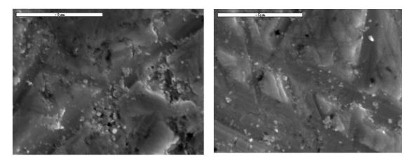
Fig. 2 Micrographs of PbTe doped with Boron sintered at 600°C (a) and 700°C (b
