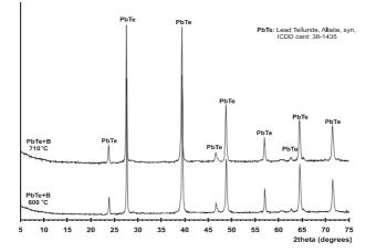
Fig. 1 X-ray diffractograms of sintered PbTe doped with Boron
