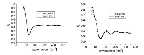
**Fig. 3** Measured (circles) and calculated (full line) far infrared reflectivity spectra of PbTe doped with Boron sintered at  $600^{\circ}$ C (a) and  $700^{\circ}$ C (b)
