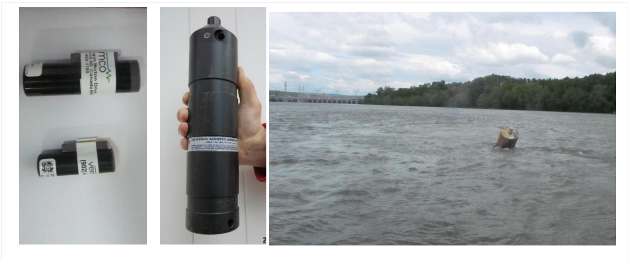
Figure 2: Equipment used for fish tagging (9 mm & 13 mm Vemco tags) - left; VR2W receiver - middle; buoy used to install receivers in the river downstream the dam – right
