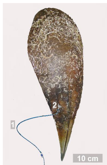
Figure 2. Pinna nobilis shell: 1—fiber-optic cable, 2—sensor attached above the heart area.
